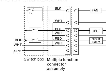
\* Under sensor status the K2 should be turned on to get high speed.
