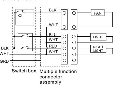
**10. For DC fan with light, night light, humidity sensor and motion sensor**
