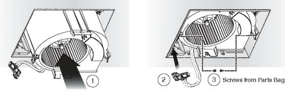
If ceiling repairs are needed, place Mask in Housing after Blower Assembly is secured. See New Construction Installation Step 6. Remove Mask before installing Grille.
