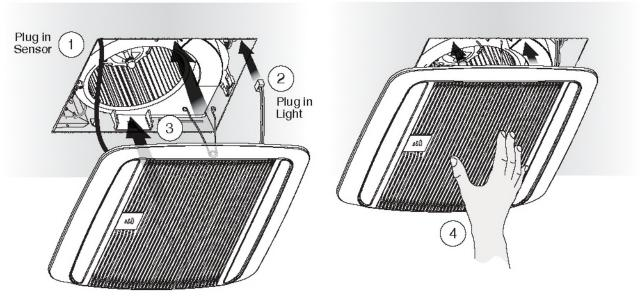
WARNING Defore servicing or cleaning unit, switch power off at service panel and lock the service disconnecting means to prevent power from being switched on accidentally. When the service disconnecting means cannot be locked, securely fasten a prominent warning device, such as a tag, to the service panel.
