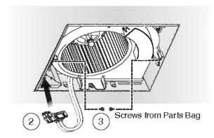
If ceiling repairs are needed, place Mask in Housing after Blower Assembly is secured. See New Construction Installation Step 6. Remove Mask before installing Grille.
