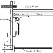
Step 6: Hang door with brackets attached on the mounting screws on to the product members. Tighten bottom screws securely. Tighten top screws (with washer) snugly allowing for future adjustment. (See illustration 5.)
