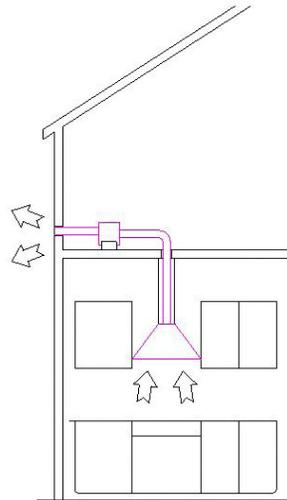
**Types of installation:** to make the installation easy, the appliance can be fixed on the wall, on the ceiling or on the floor in a horizontal position fig.2 or vertically fig. 3 to the fixing level.
