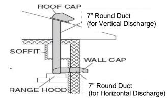
2. The range hood unit must be mounted to a liner which has the dimensions. Install the liner securely after checking that the opening size of the liner is the same as the figure below.
