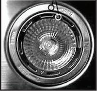
If your model uses a retaining ring light housing, twist the inner ring, using the slots and a light bulb removal tool or the edge of a small screwdriver, aligning the "OPEN" arrows, so that the retaining ring and light bulbs can be removed together.
