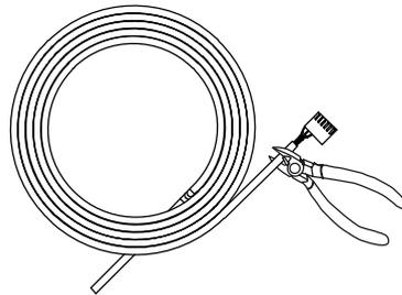
❷ Run one end of the ADA cable through the range hood wire clamp, along with the power cable, giving enough length to make the connection inside the box. Tighten the wire clamp, then strip the end of the 3 wires from provided ADA cable.
