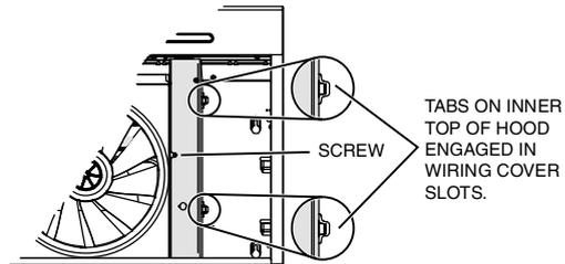
TABS ON INNER TOP OF HOOD ENGAGED IN WIRING COVER SLOTS.
