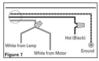
Replace the wire compartment cover and tighten screw. Make sure all wiring is securely contained within the wire compartment.
