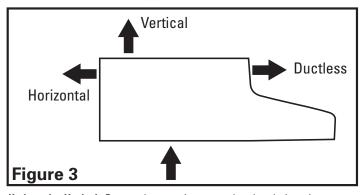
Horizontal or Vertical - Remove the apprpriate square knockout by inserting a screw driver under the edge and break the tabs holding it in place. Peel back with pliers (Figure 4).
