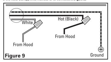
NOTE: DO NOT disconnect any wiring that has already been crimped with a wire connector from the factory.
