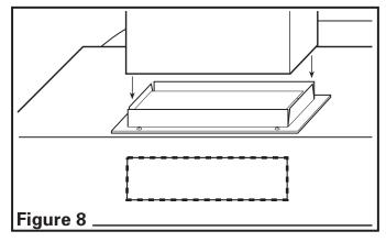
**CAUTION:** ALWAYS DUCT THE FAN TO THE OUTSIDE THROUGH A WALL OR ROOF CAP.
