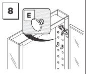
Fill remaining holes with the plugs (**E**).
