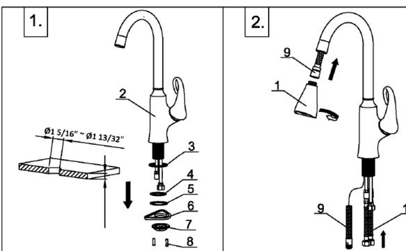
Make amounting hole. Remove parts from faucet body as shown in above diagram.
