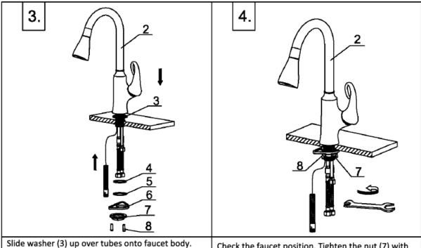
Slide washer (3) up over tubes onto faucet body. Place tubes through mounting hole and slide faucet down until it rests on mounting surface. Slide 8, 7, 6, 5 and 4 up over tubes onto faucet body.
