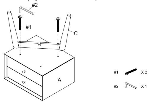
Step 2. Attach left leg (part B) to right leg (part C) and top (part A) using bolts (part #1) and allen wrench (part #2).
