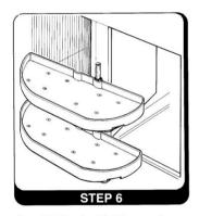
Now slide the pivot & slide assembly on shaft so it rests on the top postioner base. Your installation is now complete and should look like the illustration.
