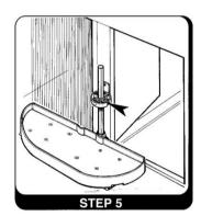
Take your pivot & slide assembly, match it over the bottom positioner base and insert the shaft through the top positioner base until the shaft bottom (open end) sets on cabinet bottom. Now tighten the set screws on both positioner bases (arrow points out top set screw). Be sure to tighten bottom positioner base set screw (not visible).
