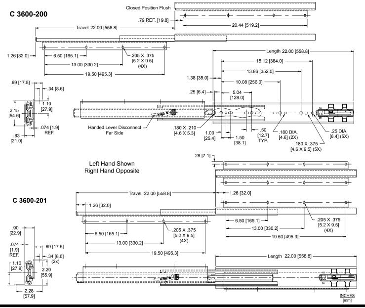
Finish Bright electro-zinc (C) plating only Mounting 3600-200: Fixed inboard bracket
